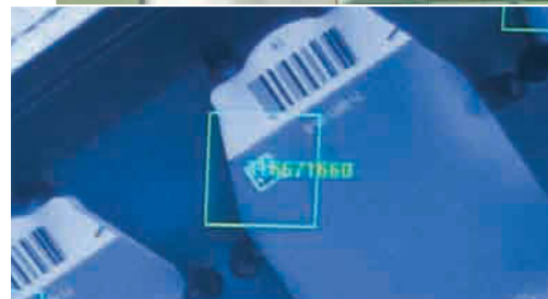
Vision system checks quality at Anderson Packaging’s production lines.
