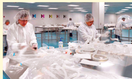
Assembly operations for single-use systems in EMD Millipore’s LEED Gold-certified clean room in Danvers, MA.
